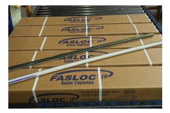
The Fasloc<sup>®</sup> resin compound is thixotropic and fast setting. This reduces viscosity during insertion and permits relatively low force and torque. The uniquely sized graded fillers assist with shredding the film, mixing the resin and, by interlocking with each other and the sidewalls of the hole, further reduce strata movement. The results are fast installation, rapid achievement of full strength, and minimum tendency for ungelled resin to drop from the holes during installation.
