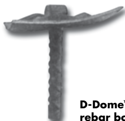
Traditional headed rebar bolt loaded to 32,000 lbs
