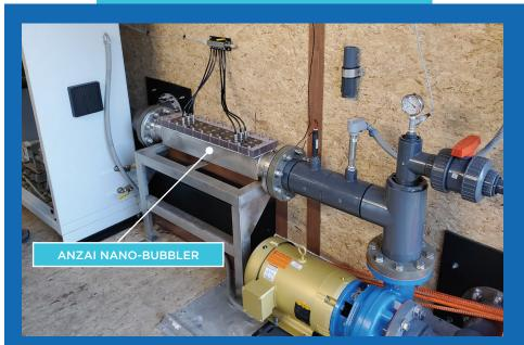
The Anzi Nano-bubbler sizes range from 1 - 1584 gpm flow rates. Pictured above is a 400 gpm unit.
